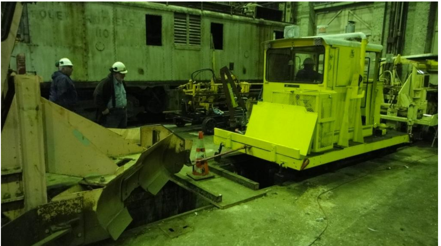
Team Tug uses the Sea Tiger as a "sea-anchor" in order to put its hydraulic system "under load" in an attempt to find the pesky hydraulic leak that only seems to materialize when the machine is pulling a heavy load.
