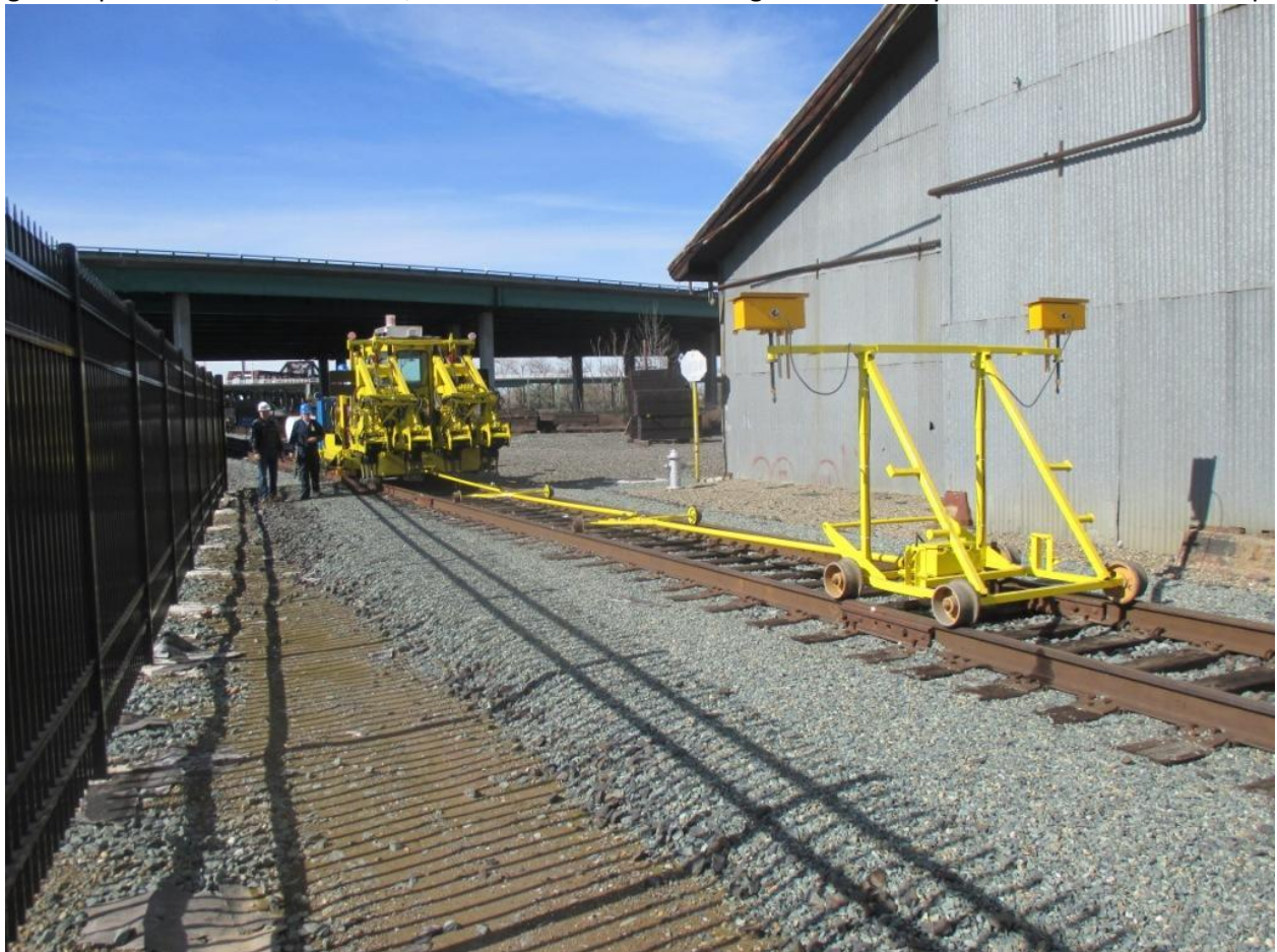
The new-old tamper with its light-reference system buggy attachment
